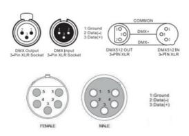
For installations where the DMX cable has to run a long distance or is in an electrically noisy environment, such as in a discotheque, it is recommended to use a DMX terminator. This helps in preventing corruption of the digital control signal by electrical noise. The DMX terminator is simply an XLR plug with a  $120~\Omega$  resistor connected between pins 2 and 3, which is then plugged into the output XLR socket of the last fixture in the chain. Please see illustrations below.
